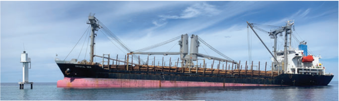
Crystal Sea aground on Greaves Reef. Note large stern trim caused through ground reaction under the bow
